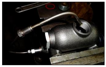
The image is a new master cylinder being held tightly in a vise. You will notice that the fitting at the bottom rear of the cylinder has been installed onto the new master cylinder. SEE THE BOTTOM LEFT OF THE MASTER CYLINDER. This fitting is about 1" long and has a male thread which screws into the master cylinder on one side and has a female tread on the other side where the brake line from the three way fitting on the frame rail screws into.
